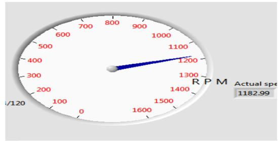
Fig.5 Measurement of speed using D I/O
