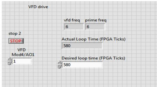
Fig.4 Prime mover speed control
