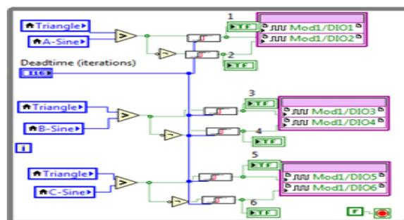
Fig.3 LabVIEW VI for sine PWM
