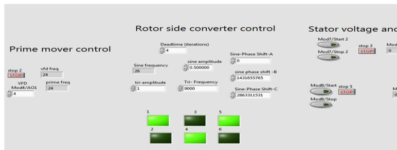
Fig.10 Front panel of LabVIEW FPGA VI for DFIG control
