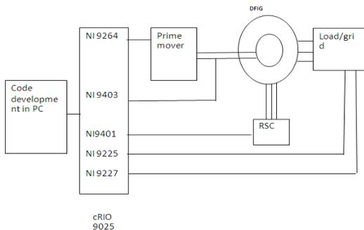
Fig.8 Implementation of DFIG control using NI LabVIEW platform
