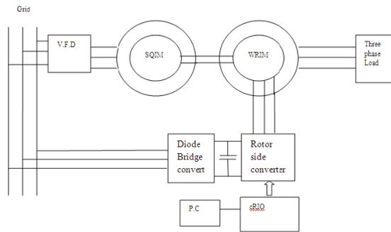
Fig.7 Block diagram of DFIG system
